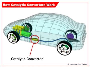
Removes carbon monoxide from exhaust fumes:
